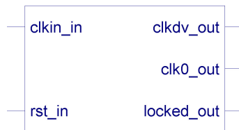
Figure A.151 Resulting top level RTL symbol for the synthesized DCM.
